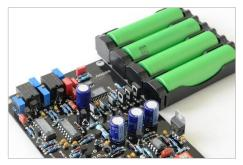
The electronics has been developed especially for our turntable. It is a closed loop controller which keeps the speed of the motor constant. The feedback of the brushless DC-motor is compared with an extreme precise reference voltage, which makes the drive unit significant more accurate than a pll-system with quartz controlled oscillator. The outstanding feature of the TTT-Compact II is the battery based power supply
