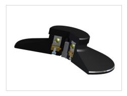
Unlike most turntables, for the TTT is the clamp part of the main concept. It defines the contact between the record and the carefully designed mat and platter. The clamp attaches a (very little) deformation to the record-label to make sure the record touches the mat surface all over. This deformation is fully guided between shape and counter shape. Even the hold-down-force is defined by a spring-loaded mechanism and is independent of the torque you are tightening the
