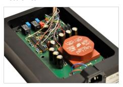
The electronics has been developed especially for the TTT. It is a closed loop controller which keeps the speed of the motor constant. The feedback of the brushless DC-motor is compared with an extreme precise reference voltage, which makes the drive unit significant more accurate than a pll-system with quartz controlled oscillator. This preciseness can only be reached by using circuits with a perfect temper-
