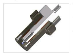
The bearing of the TTT is our homage to traditional crafts-manship. The approved construction is known since more than 50 years in the industry, while we have brought the realization and finish to a new level by combining it with traditional knowledge of our watchmaker. The main shaft is made of hard chrome plated carbon tool steel. Its surface has been hand polished step by step with basswood and diamond-paste. The shaft runs in two sintered bronze bush-
