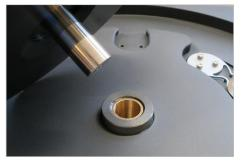
The bearing of the TTT-Slim II is our homage to traditional craftsmanship. The approved construction is known since more than 50 years in the industry, while we have brought the realization and finish to a new level by combining it with traditional knowledge of our watchmaker. The main shaft is made of hardened carbon tool steel. Its surface has been hand polished step by step with basswood and diamond-
