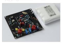
The electronics has been developed especially for our turntable. It is a closed loop controller which keeps the speed of the motor constant. The feedback of the brushless DC-motor is compared with an extreme precise reference voltage, which makes the drive unit significant more accurate than a pll-system with quartz controlled oscillator. The outstanding feature of the TTT-Slim II is the battery based power supply with Li-Ion
