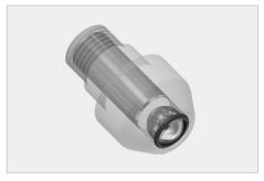
The spikes look quite common from outside, but the secret of the decoupling and leveling mechanism is inside. The spikes make the turntable standing on balls, keeping it in position by a small rubber element. This keeps horizontal vibration of the ground away efficiently. The leveling mechanism is a combination of a machined thread with a high precision sliding fit. This makes leveling of the unit easy, secure and precise, while
