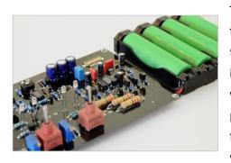
The electronics has been developed especially for our turntable. It is a closed loop controller which keeps the speed of the motor constant. The feedback of the brushless DC-motor is compared with an extreme precise reference voltage, which makes the drive unit significant more accurate than a pll-system with quartz controlled oscillator. The outstanding feature of the TTT-Slim is the battery based power supply with Li-Ion accumulators. The peak capacity is higher than
