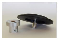
The bearing of the TTT-Slim is our homage to traditional craftsmanship. The approved construction is known since more than 50 years in the industry, while we have brought the realization and finish to a new level by combining it with traditional knowledge of our watchmaker. The main shaft is made of hardened carbon tool steel. Its surface has been hand polished step by step with basswood and diamond-
