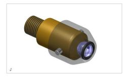
The spikes look quite common from outside, but the secret of the decoupling and leveling mechanism is inside. The spikes make the turntable standing on balls, keeping it in position by a small rubber element. This keeps horizontal vibration of the ground away efficiently. The leveling mechanism is a combination of a machined thread with a high precision sliding fit. This makes leveling of the unit easy,
