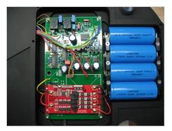
The electronics has been developed especially for our turntable. It is a closed loop controller which keeps the speed of the motor constant. The feedback of the brushless DC-motor is compared with an extreme precise reference voltage, which makes the drive unit significant more accurate than a pll-system with quartz controlled oscillator. The outstanding feature of the TTT-Compact is the battery based power supply with LiFePo accumulators, using nano-technology. The
