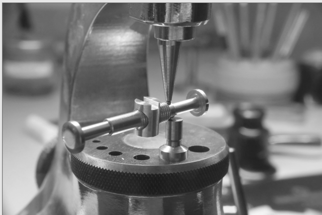
Assembling vernier for azimuth
