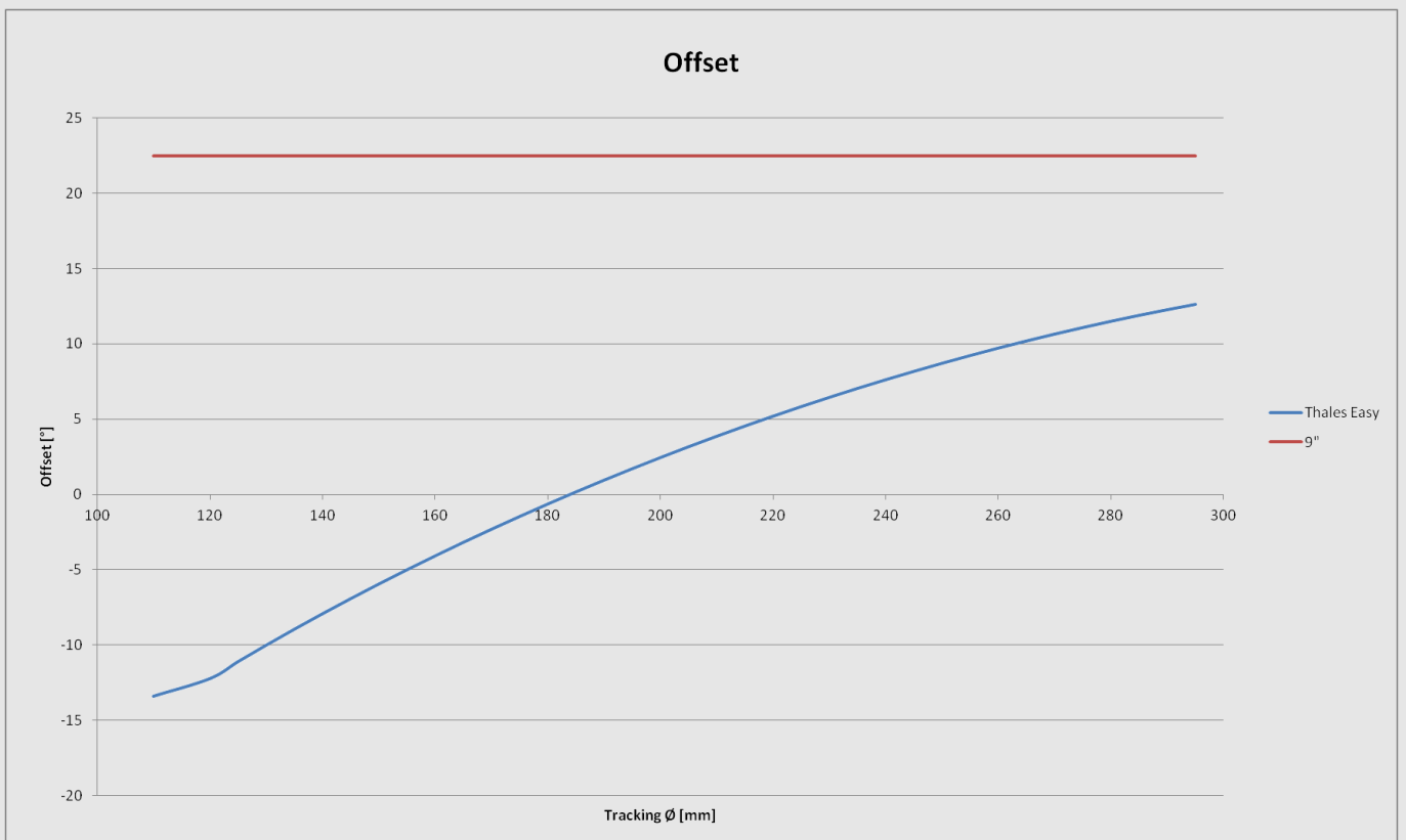
The variable offset angle of the Thales Easy compared with the fixed angle of a traditional 9" tonearm
